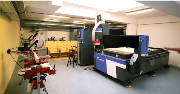
Wood workshop with large-format CNC milling machine for professional woodworking.
